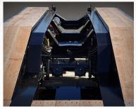
Remove the center bogie section to create a low boom well that is great for hauling excavators. The 4-point lift system makes it easy to convert.
